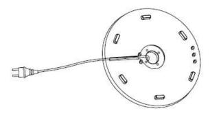
Step 3: Place the power cord plug through base, middle pole and top pole. Connect the powercord plug to the socket in the heater head.
