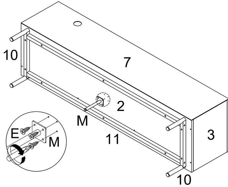
Please note that hardware M has a **Plastic adjuster** at the bottom to unscrew and adjust the height of hardware M if necessary.
